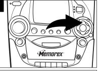
When the desired track number blinks in the display, within five seconds, press the Play/Pause (►II) button. Playback will begin on the track you selected.
